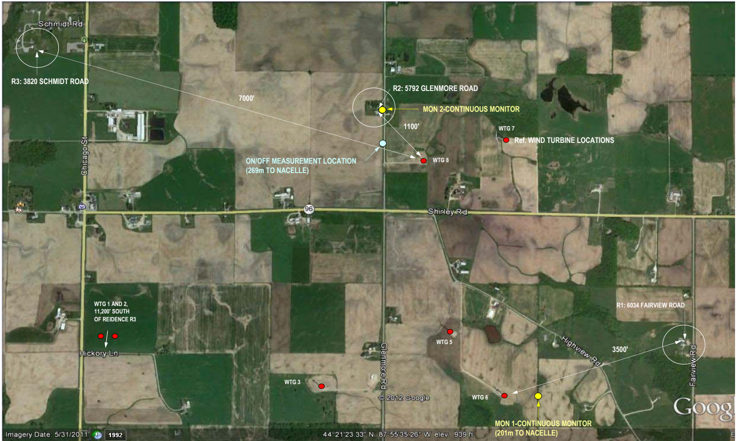
Figure 2.1: Aerial view showing sound survey locations
